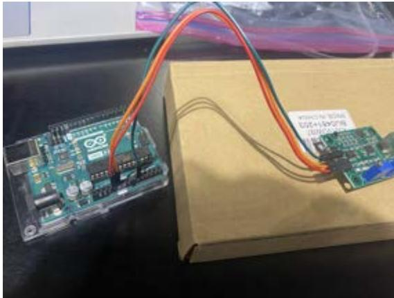
This is what the pH probe looks like connected to the arduino. We connect the arduino to the laptop in order to compile the code onto it.
