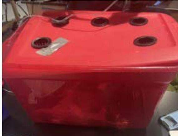
This is what our bin looks like with the holes drilled and the net pods placed on the top, once we have our robotic system which will drill out a section for the probe to access the water. As you can see the tube coming from the left side of the bin; this is the water pump hooked up to our airstone which bubbles oxygen into our water and will allow our plants to prosper.
