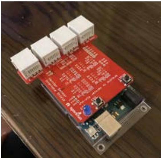
We have the vernier interface shield and the red board and although connecting sensors is way easier the shield although we run into another problem where the Vernier interface shield does not allow us access to the SDA and SCL ports on the arduino which we need for the motors.
