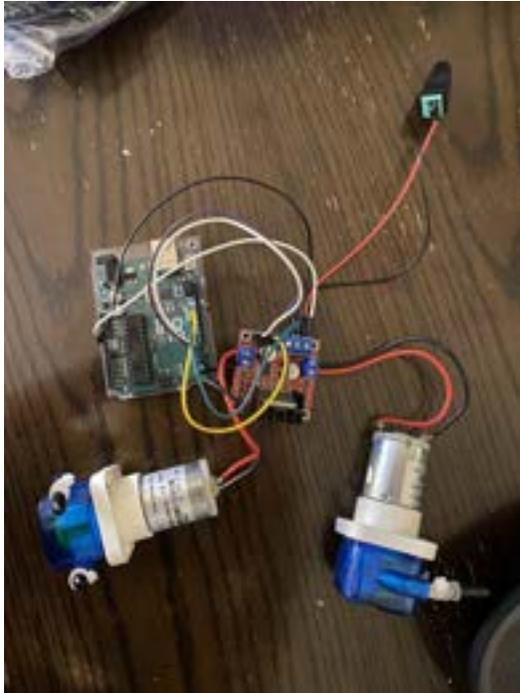
This is our setup for the motors connected to the Arduino. In the middle you see our DC motor controller and it is what connects our pumps to our arduino. It is a L298N motor controller. Yesterday I sutured the motors to the motor controller using a suture.
