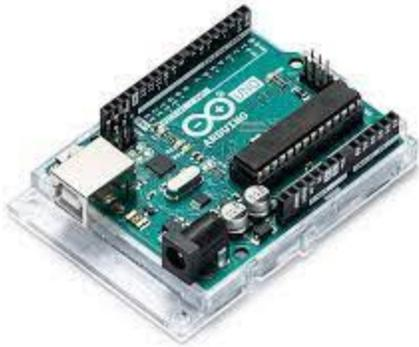
Using an arduino we are able to connect it to a pH meter as well as a peristaltic pump. Assembling Hardware is the first step so we will need to set the pH circuit and pumps to 12C where each device is assigned a unique 12C address.
