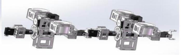
Figure 3.13: Two drones attached together as drawn on Fusion 360
