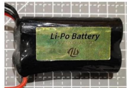
Figure 3.17: Servo Battery
