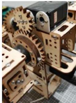
Figure 3.6: The x-axis gear with respect to the rest of the drone
