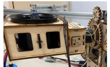
Figure 3.1: Two boxes which attaches the ducted fan to the rod.
