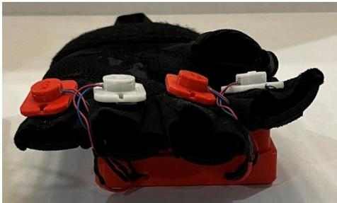
*Figure 2: O.D.U.S.+ Glove with Vibration Motors and the Raspberry Pi Zero W*
