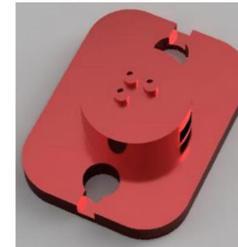
Figure 4: 3-D Render of the Front Vibration Motor Case
