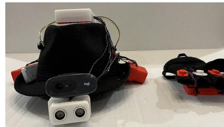
Figure 8: The completed O.D.U.S.+ , with all the ultrasonic sensors, the vibration motors, the Raspberry Pi's, and the camera, all in working order
