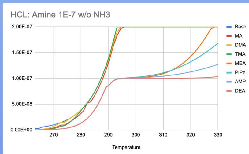
Fig 7. Amines at 1E-7, no NH3; MEA and PiPz are part of lower curves, base, MA, and DMA curves are higher
