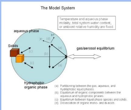
Fig 2. Visual of how E-AIM Model System functions, partitioning across aqueous, organic, gas, and solid phases
