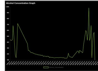
In the above line chart, the green line represents the values the MQ3 alcohol sensor outputs. Each peak in the graph at the values at 690, 710, and 990 represent spikes due to the spraying of alcohol.
