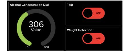
This is the user configuration dashboard. The client can view the latest value detected by the sensor through the alcohol concentration dial as well as whether or not someday is sitting in the driver's seat of the car through the weight detection toggle. The text toggle will also display if an alert has been sent.
