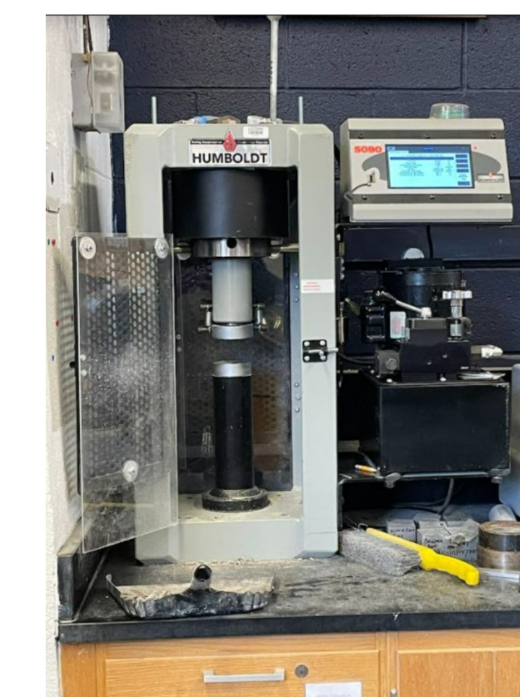
Left: Assembled cubic molds, UHPC mixture, and machine used for grinding the samples. Above: Humboldt Compression Machine used for testing.
