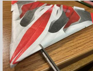
Figure 2. Performing one of the four cuts on the leading-edges.
