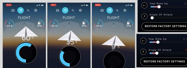
Figure 3. From left to right, setting throttle at 60% for takeoff, reducing the throttle to 35% for cruising, and abruptly reducing the throttle to 7% for a powered descent.
