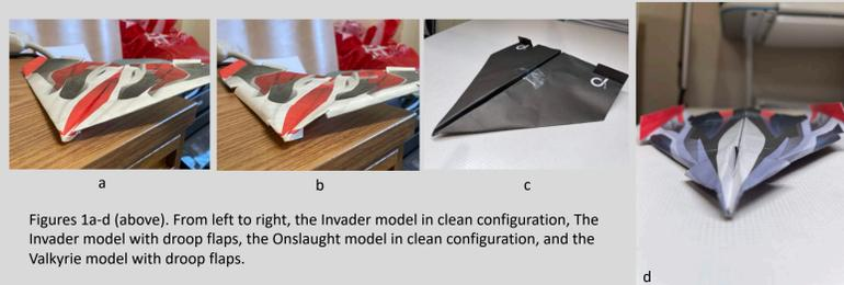
Figures 1a-d (above). From left to right, the Invader model in clean configuration, the Invader model with droop flaps, the Onslaught model in clean configuration, and the Valkyrie model with droop flaps.
