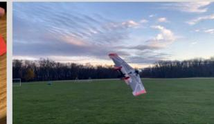
Figure 4. The Valkyrie model in action. Out of the three models, the Valkyrie has the largest wing area but the lowest aspect ratio.
